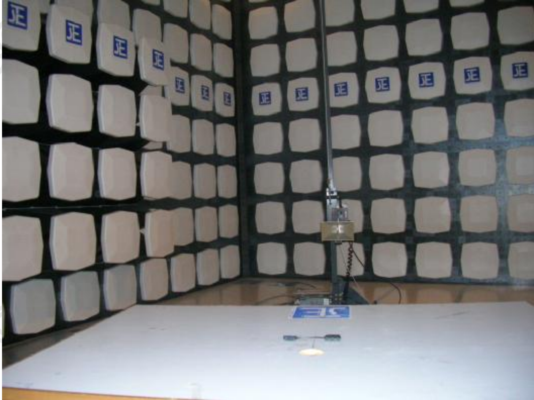
Measurement of Radiated Emission Test Set Up
