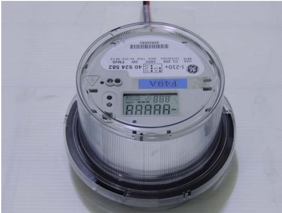
Photograph 7: Set-up for Radiated Emission, EUT Configuration Z-Axis
