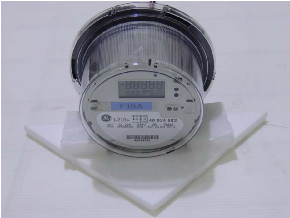
Photograph 5: Set-up for Radiated Emission, EUT Configuration X-Axis
