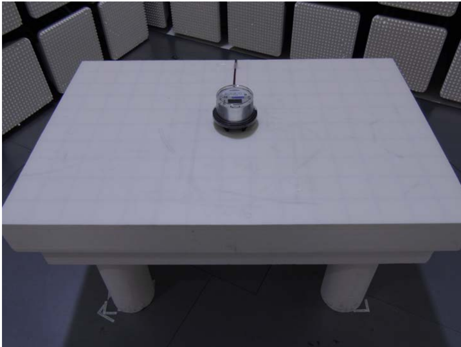
Photograph 3: Set-up for Radiated Emission of Transmitter, Front View
