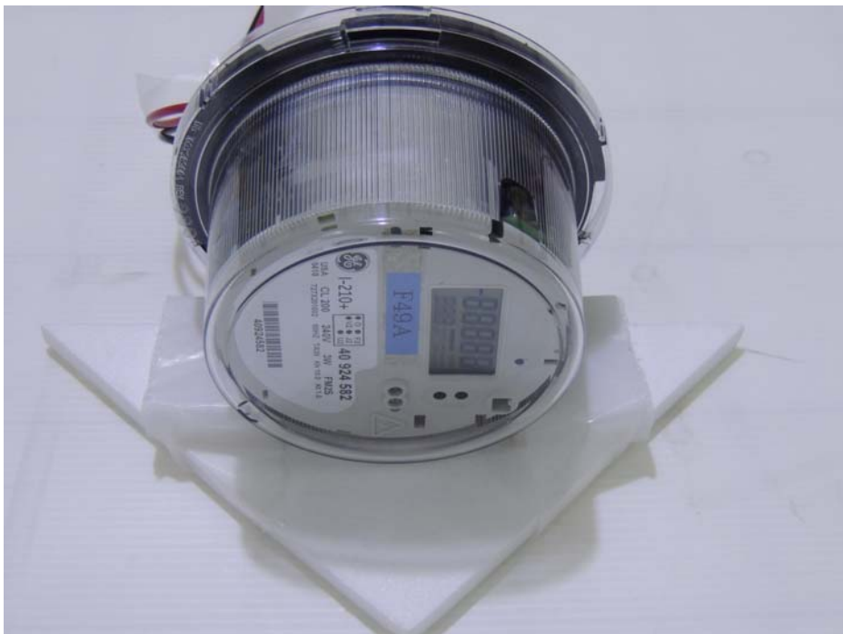
Photograph 6: Set-up for Radiated Emission, EUT Configuration Y-Axis
