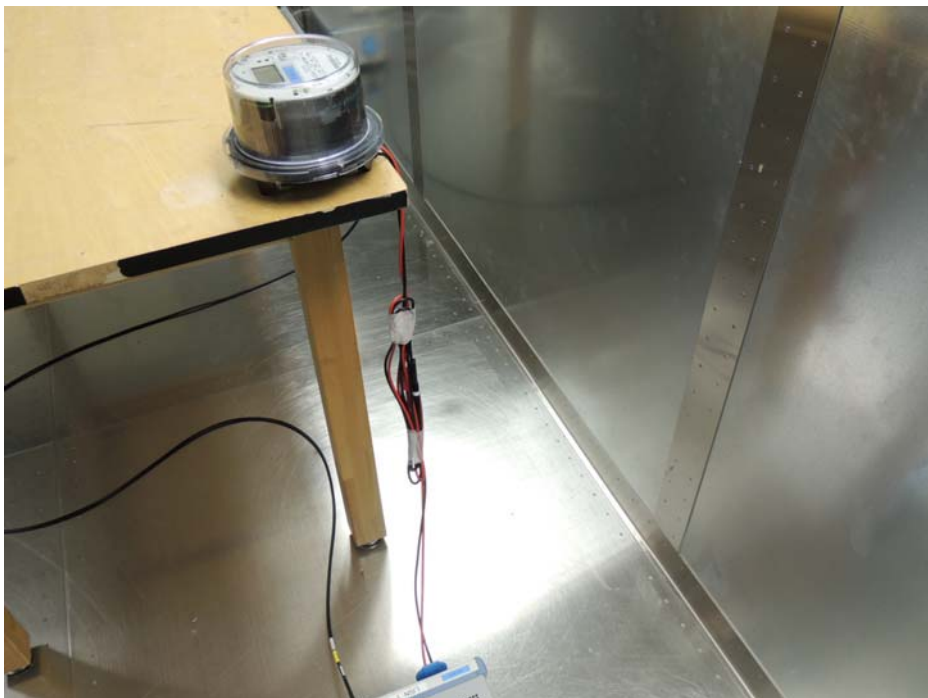
Photograph 8: Set-up for AC Power Line Conducted Emission of Transmitter
