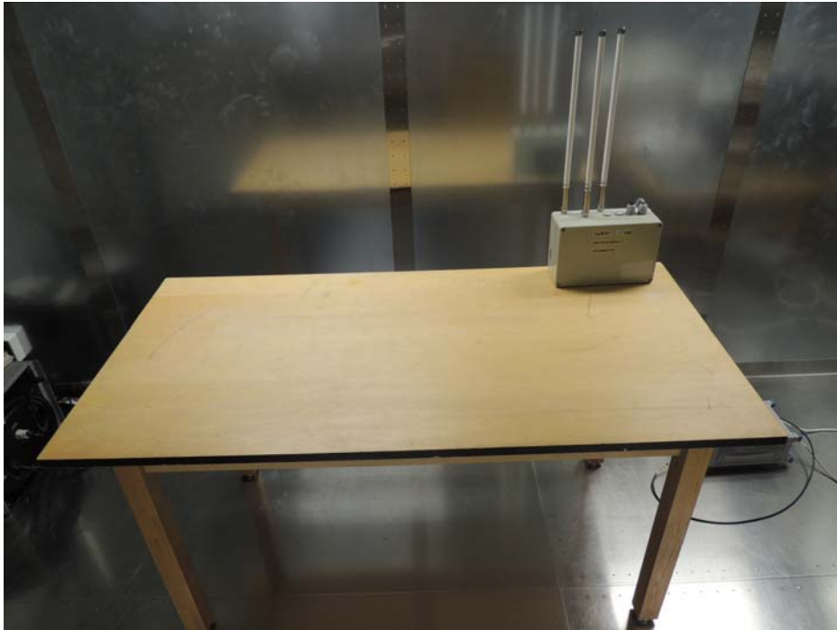
Photograph 3: Set-up for AC Power Line Conducted Emission of Transmitter, Rear View
