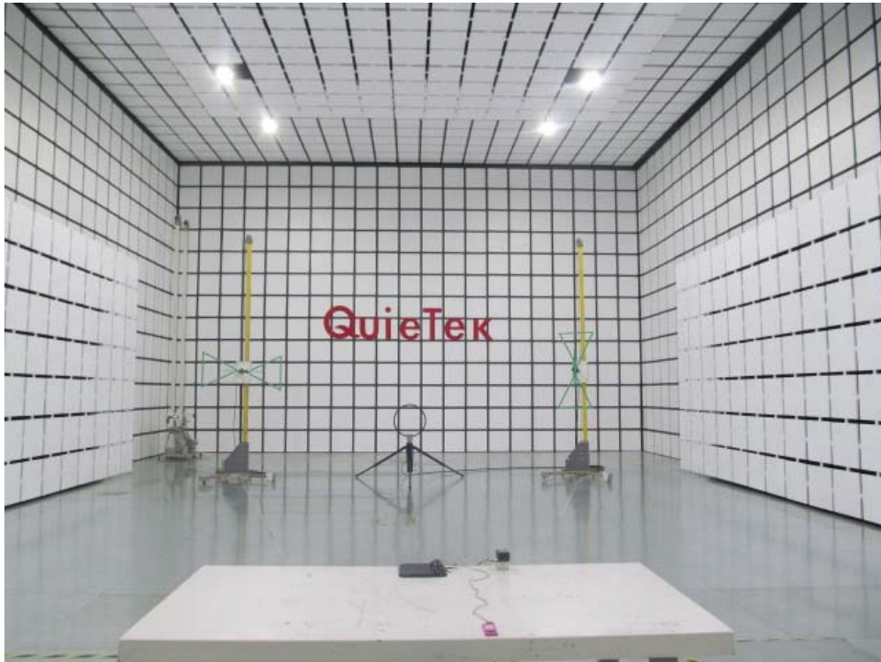
Description: Radiated Emission Test Setup for Below 30MHz
