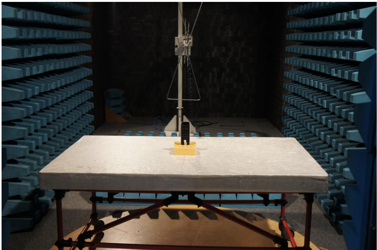
Picture 5: test setup radiated emission test 30 MHz - 1 GHz, premeasurements
