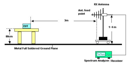
$\hbox{(C) Radiated Emission Test-Up Frequency Above 1GHz}\\$
