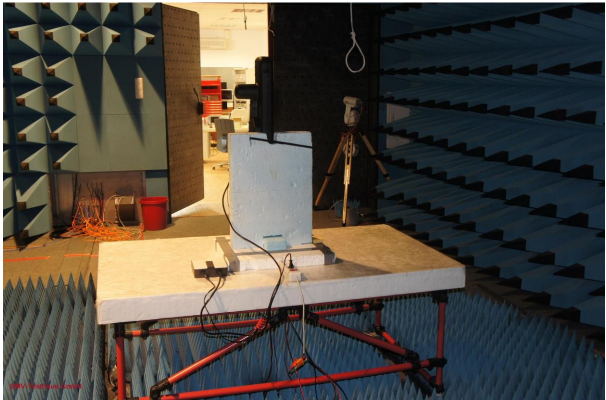
Picture 13: EUT test setup radiated emissions > 1GHz - rear view
