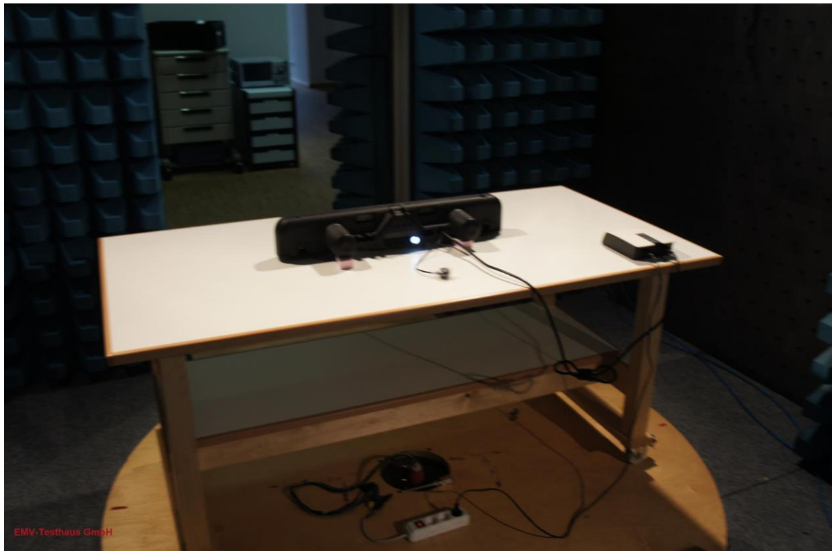
Picture 7: test setup radiated emissions 9 kHz - 30 MHz, CDC, rear view
