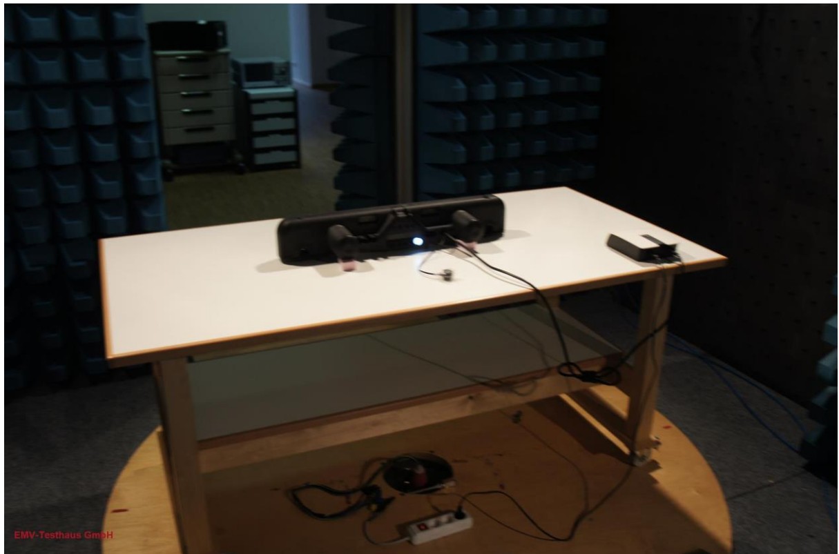
Picture 9: test setup radiated emissions 30 MHz - 1 GHz, CDC, rear view
