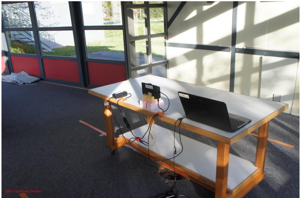
Picture 11: test setup radiated emissions, OATS, rear view
