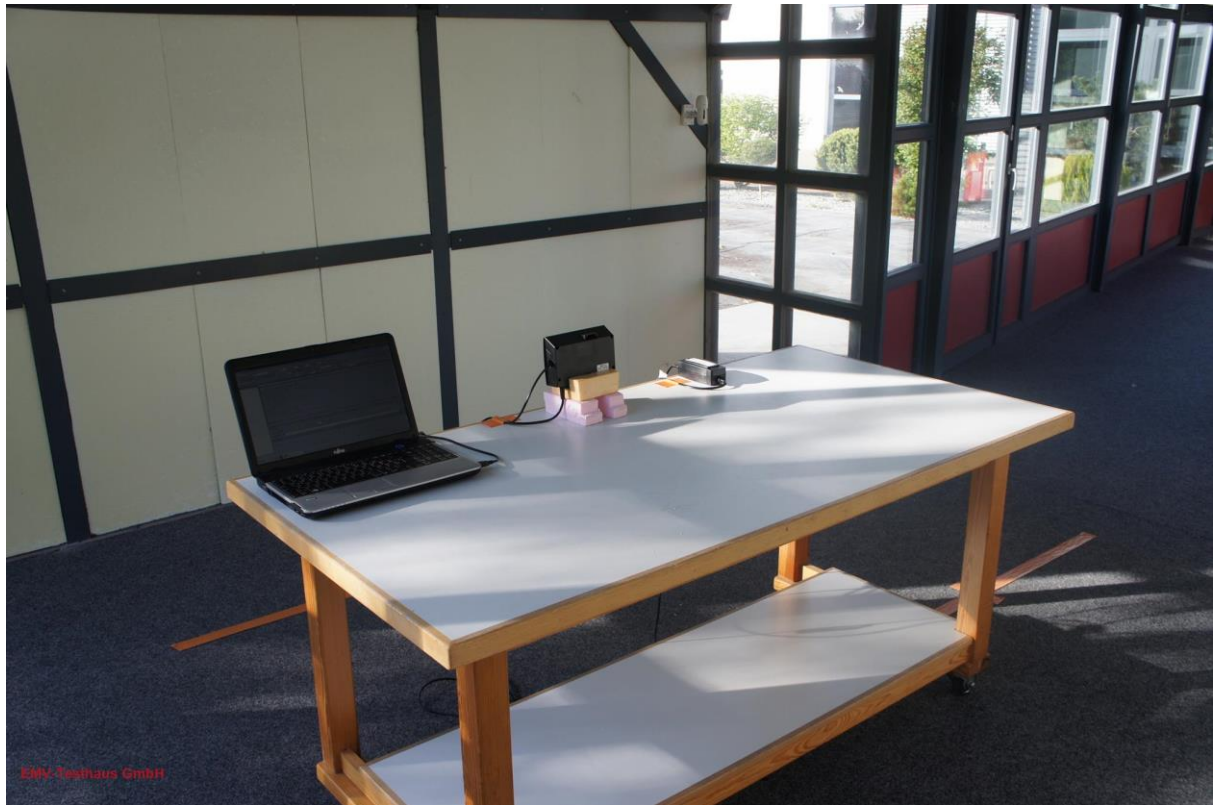
Picture 10: test setup radiated emissions, OATS, front view
