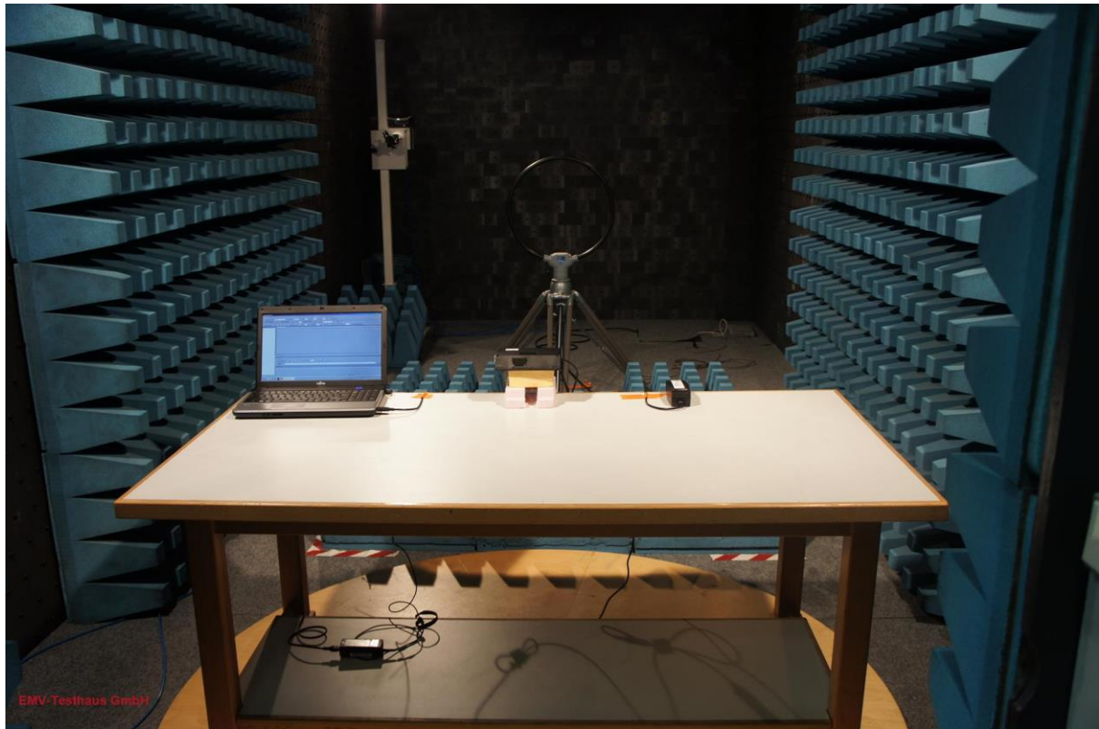
Picture 6: test setup radiated emissions 9 kHz - 30 MHz, CDC, front view
