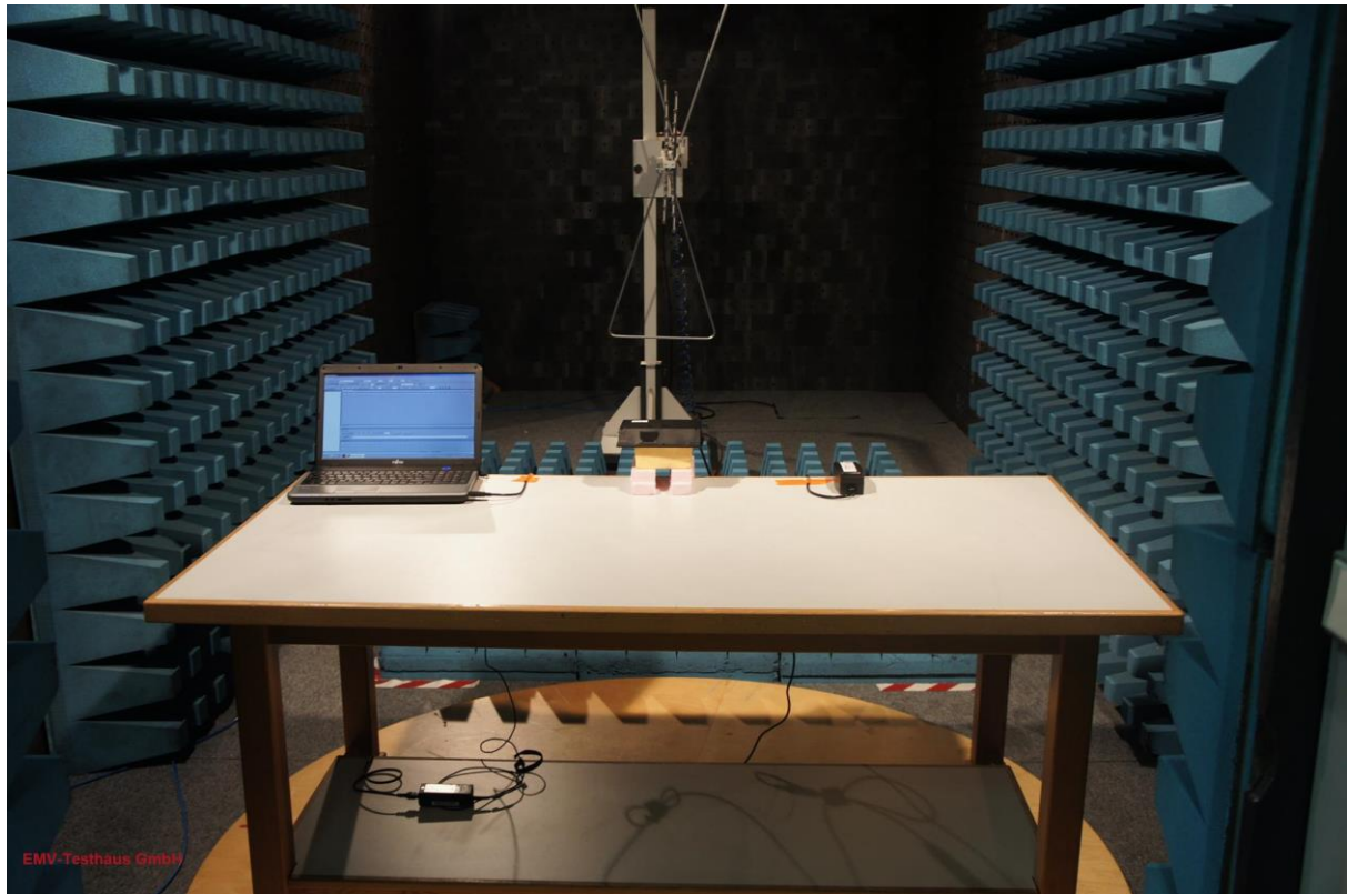
Picture 8: test setup radiated emissions 30 MHz - 1 GHz, CDC, front view
