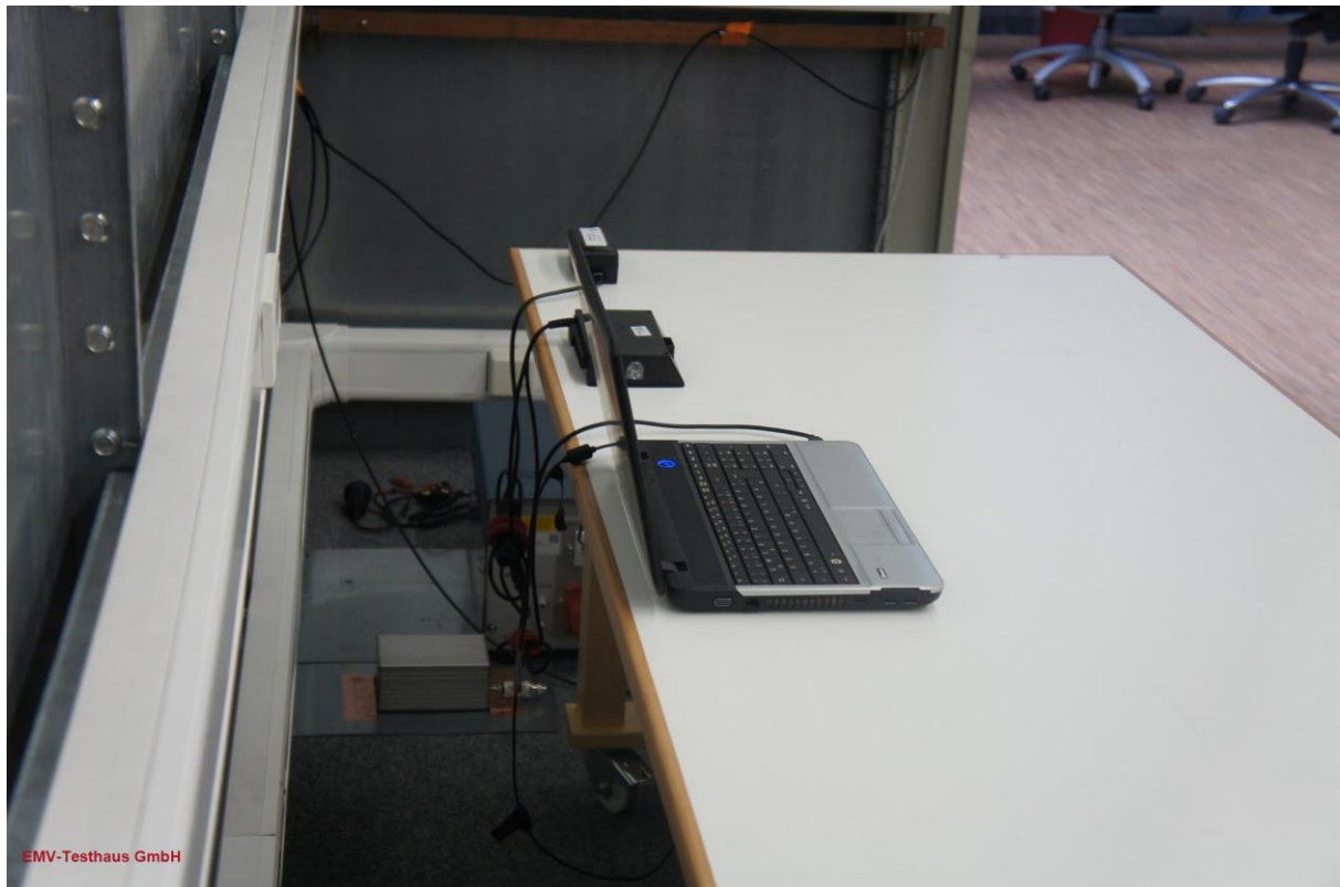
Picture 5: test setup AC power line conducted emissions, rear view
