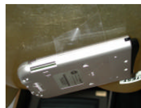
Fig. 10 Body SAR Test Setup (reverse shirt pocket)
