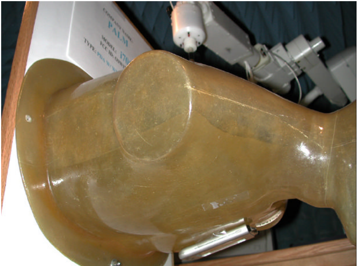
Fig. 8 Test Setup of EUT in operating position with the source of significant emissions (antenna) touching the phantom.
