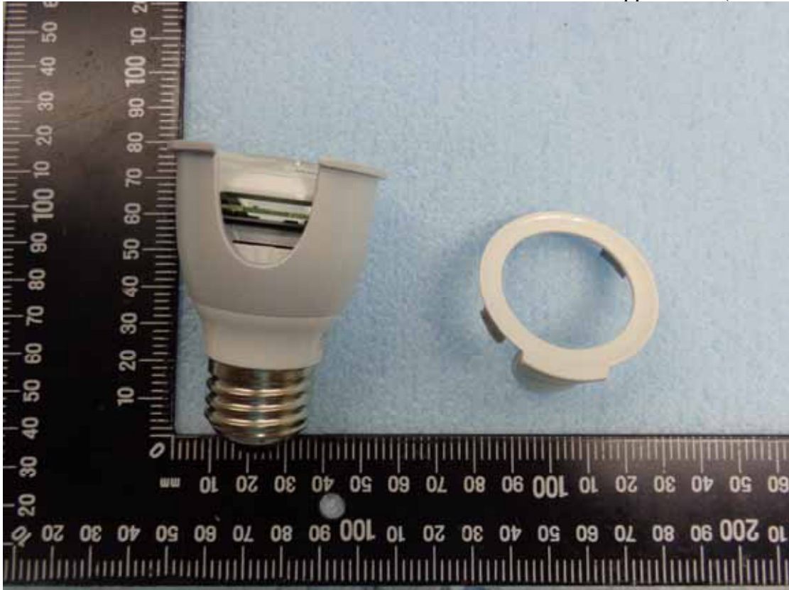
Figure 1 General Appearance (Cover Remove)
