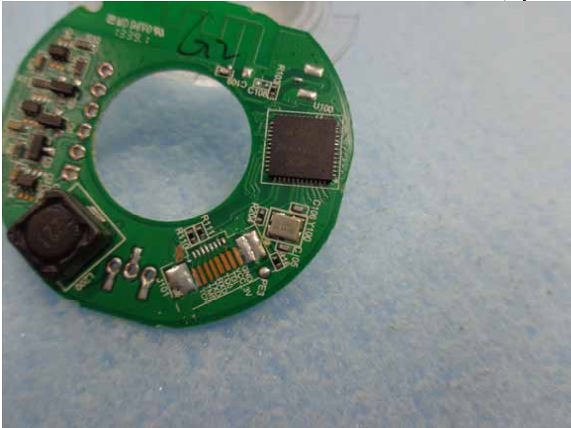
Figure 7 Wireless Board (Crystal Oscillator)
