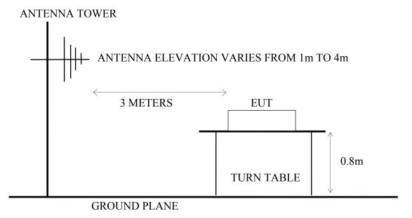
4.2.3. No. 1 3m Semi-Anechoic Chamber Setup Diagram (Test distance: 3m) for above 1GHz
