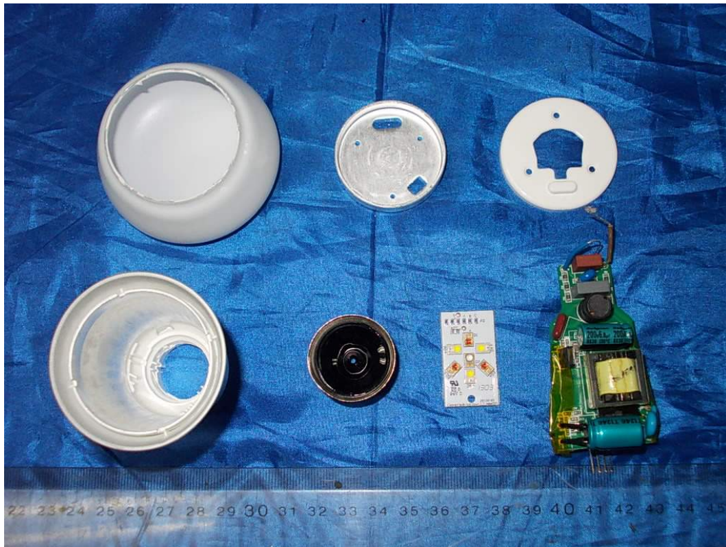
FIGURE 2 LED LAMPS (M/N: 9290002265) COVER REMOVED
