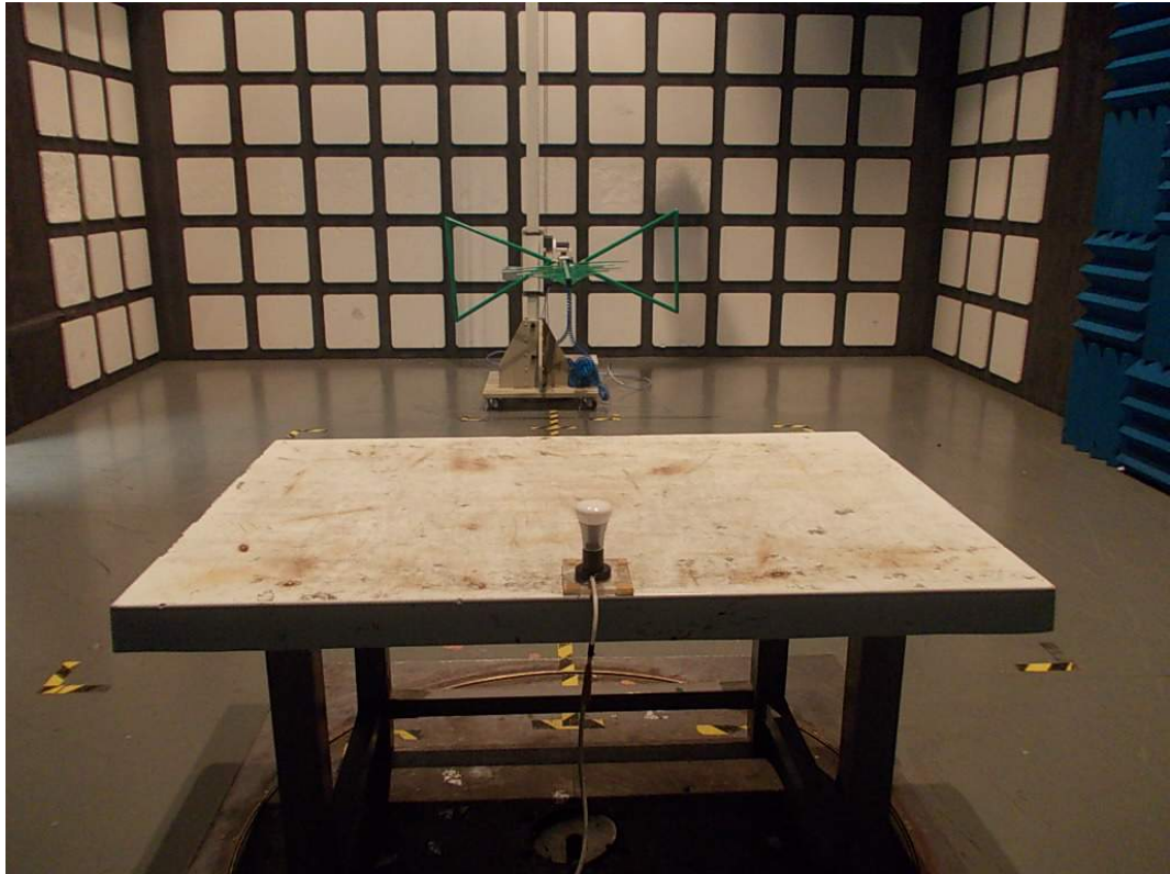
RADIATED EMISSION TEST (BELOW 1GHZ)
