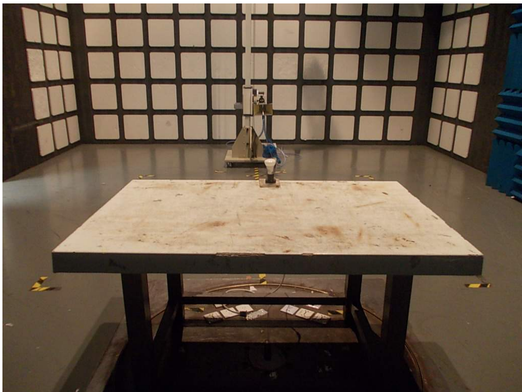
RADIATED EMISSION TEST (ABOVE 1GHZ)
