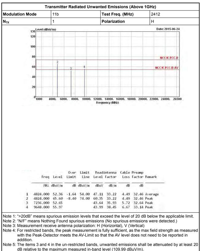
Note 6: No level of unwanted emissions exceeds the level of the fundamental emission.
