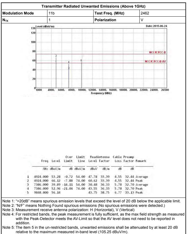
Note 6: No level of unwanted emissions exceeds the level of the fundamental emission.
