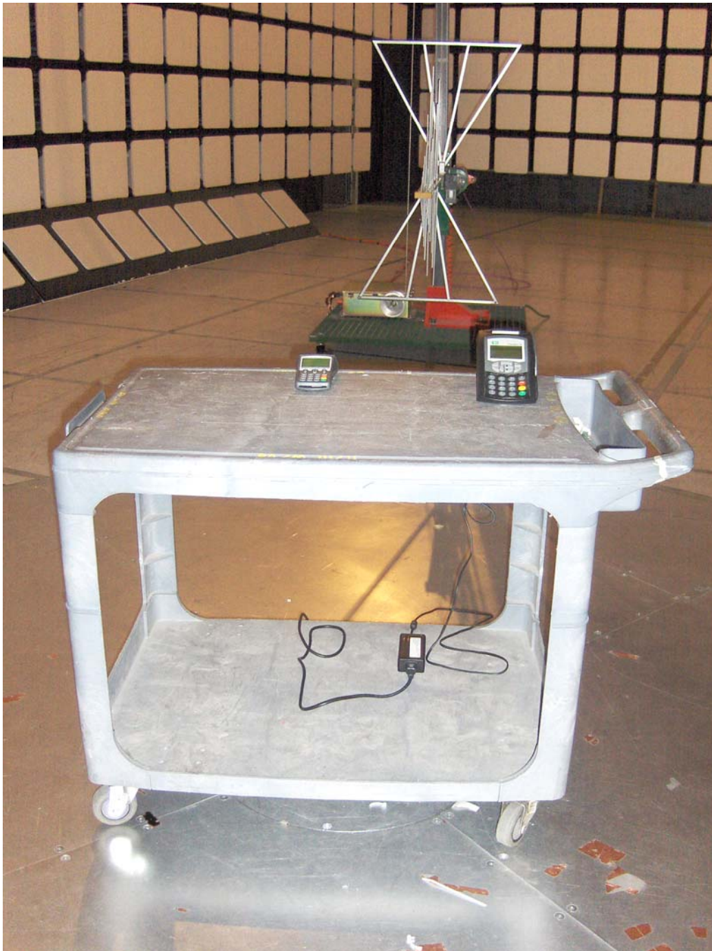
Radiated Emission at 3 m Distance (30 – 1000 MHz)
