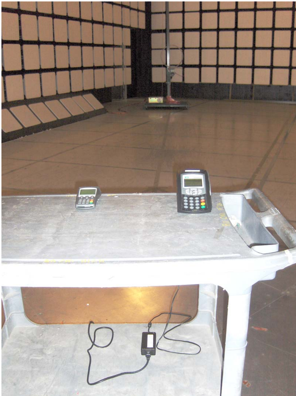
Radiated Emission at 10 m Distance (Below 30 MHz)
