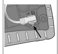
To take of the cable, press the flap N°1 and pull the cable N°2.
