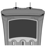
NBS7250 is maintained by a notch situated on its front side and two clips on the back side. In order to install it on its base, first introduce the front side of the equipment and then, make a press on its back side until hearing the locking noise. In order to remove it from the base, remove the two clips one after the other while pulling up the equipment
