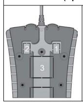
The Ethernet cable is optional. The path is through the hole(2). The opening in the table must be 14mm diameter.
