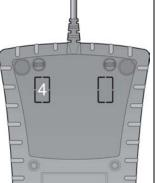
The back cover may be opened as mentioned as 4 in order to have a path for Ethernet cable. (option) The descriptions, illustrations and characteristics in this document are only given for information and not contractually binding. NBS Payment Solutions – the Division of NBS Technologies Inc. reserves the right to make any alterations without prior notice. All rights of reproduction, adaptation, execution, and translation reserved in all countries.
