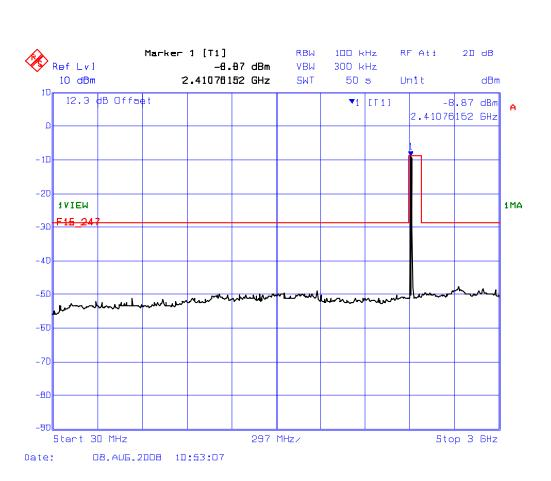
Plot 5.8.4.2.1.1. Spurious RF Conducted Emissions Transmitter Frequency: 2412 MHz
