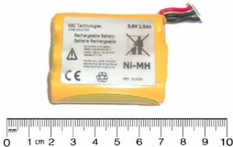
< Rechargeable Ni-MH battery (3.6V, 1.5 Ah) >
