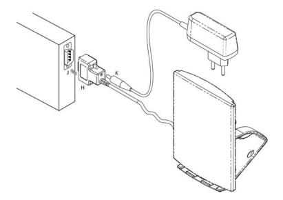
Connect the power adapter (jack **K**) to the connector **H**. Connect the other end of the RS232 cable (port **H** to port **J**). **Screw** connector **H** firmly to the equipment.
