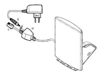
Connect the power adapter (jack **K**) to the connector **H**. Connect the other end of the RS232 cable (port RJ11 **L**). Connect the power adapter to the incoming power supply socket. Once installed, **leave the NBS1200 on permanently**.
