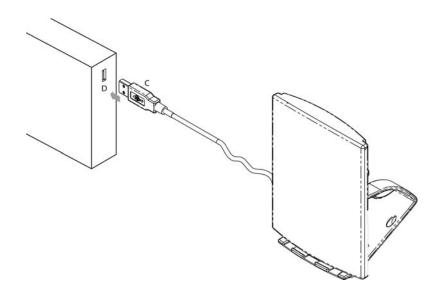
Connect the end of the USB cable (port **C**) to the equipment (port **D**). Once installed, **leave the NBS1200 connected at all times**.
