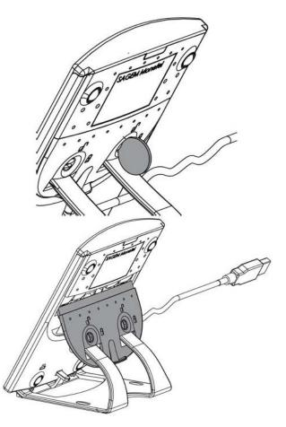
3. Slide the access cover down the frame to clear it fully
