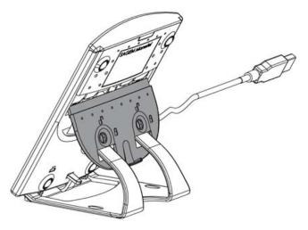
5. Close the access cover, and then move the quarter-turn notches back to the horizontal position, while pressing the access cover down firmly.
