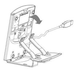
4. Fix the top of the SAM access cover into the guard as shown in the figure opposite
