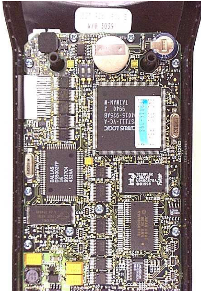
Freedom II-D with a Research in Motion RIM802D Transmitter DataTAC Modem: rear of display
