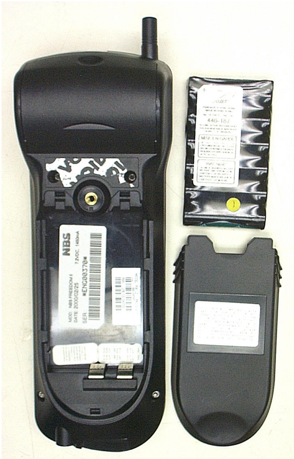
Battery and compartment
