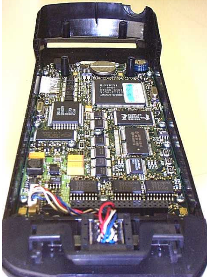
Freedom II-D with a Research in Motion RIM802D Transmitter DataTAC Modem: Rear of display and keyboard
