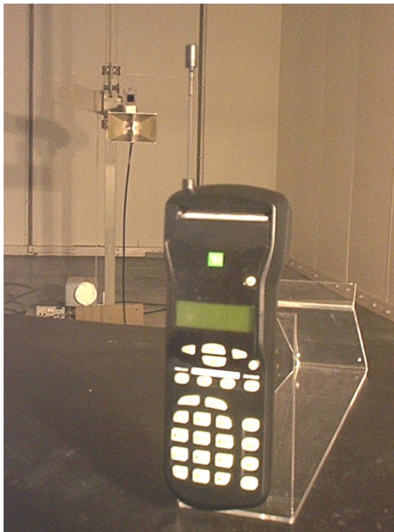
Spurious Emission Testing (for frequencies above 1 GHz)
