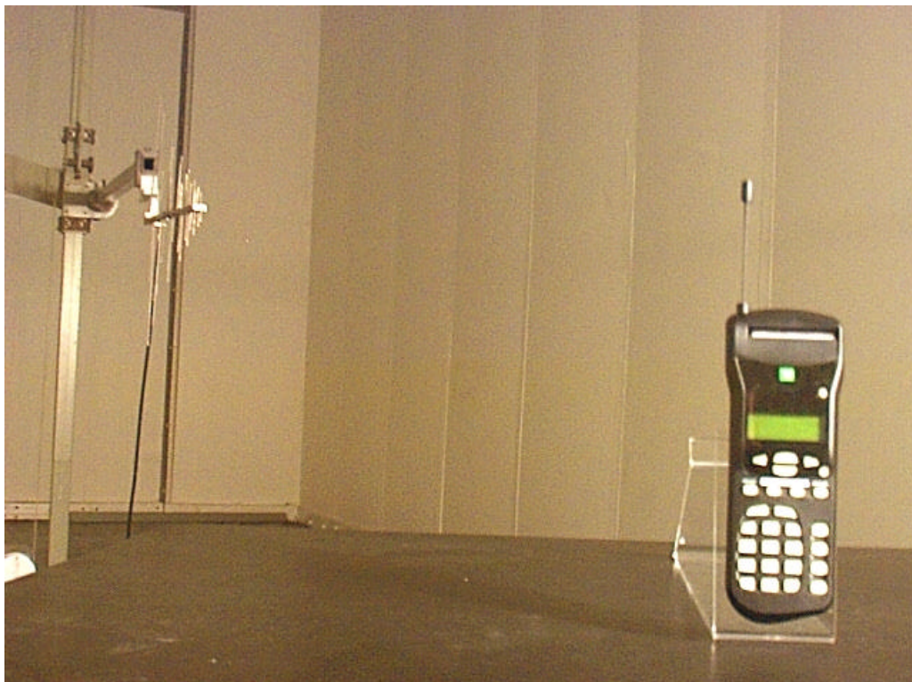
Spurious Emission Testing (frequency range: 200 MHz – 1GHz)
