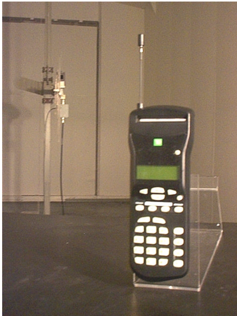
Field Strength of Spurious Radiation measurement in OATS
