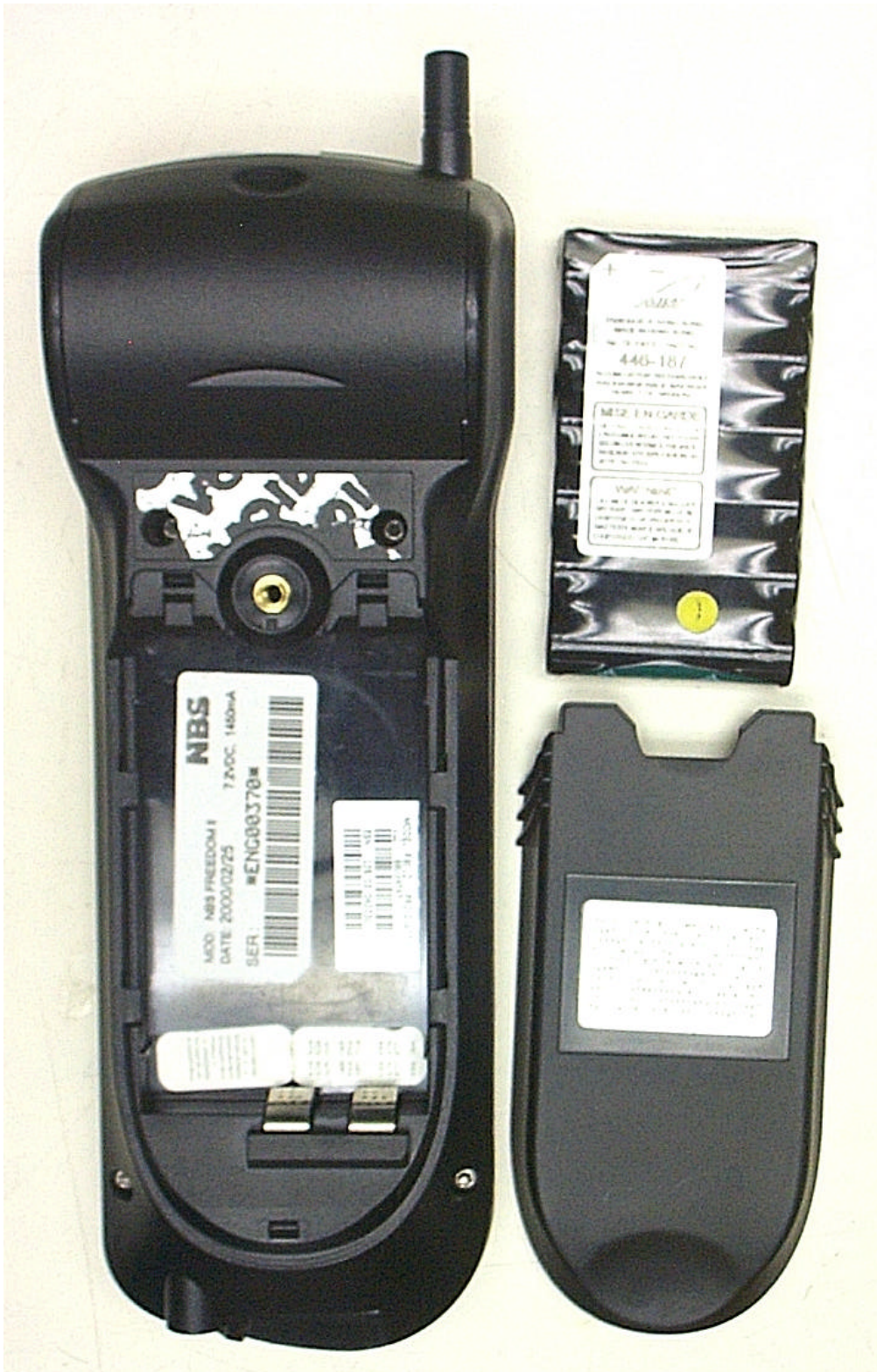
Battery and compartment
