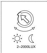
The chosen light response threshold can be infinitely from approx. 2-2000lux. Turn it fully anti-clockwise to select dusk- to-dawn operation at about 2 Lux. Turn it fully clockwise to select daylight operation at about 2000lux. The knob must be turned fully clockwise when adjusting the detection zone and performing the walk test in daylight.
