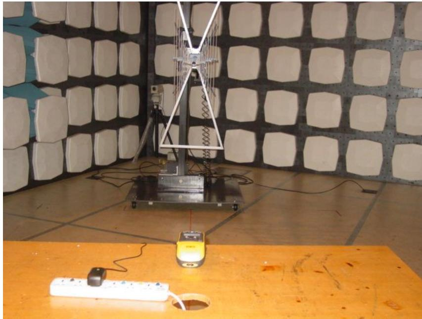
**FCC Radiated Emission Test Setup (Reading)**
