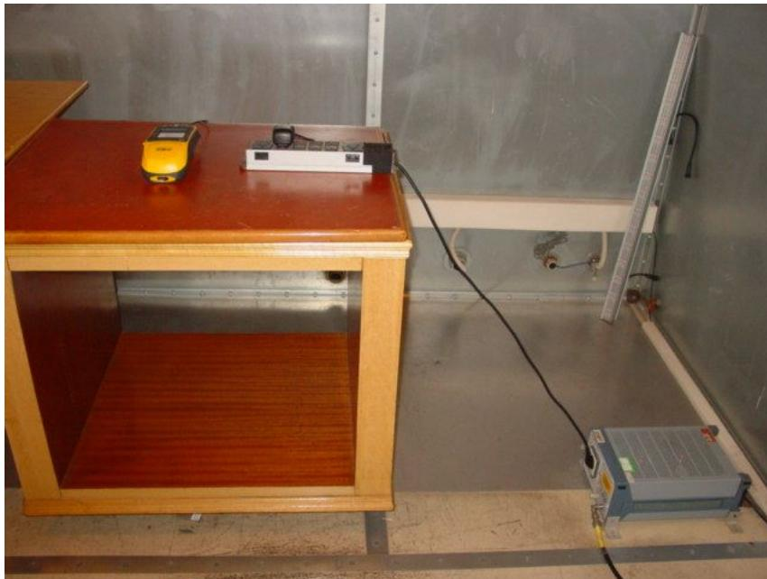
**FCC Conducted Emission Test Setup (Reading)**
