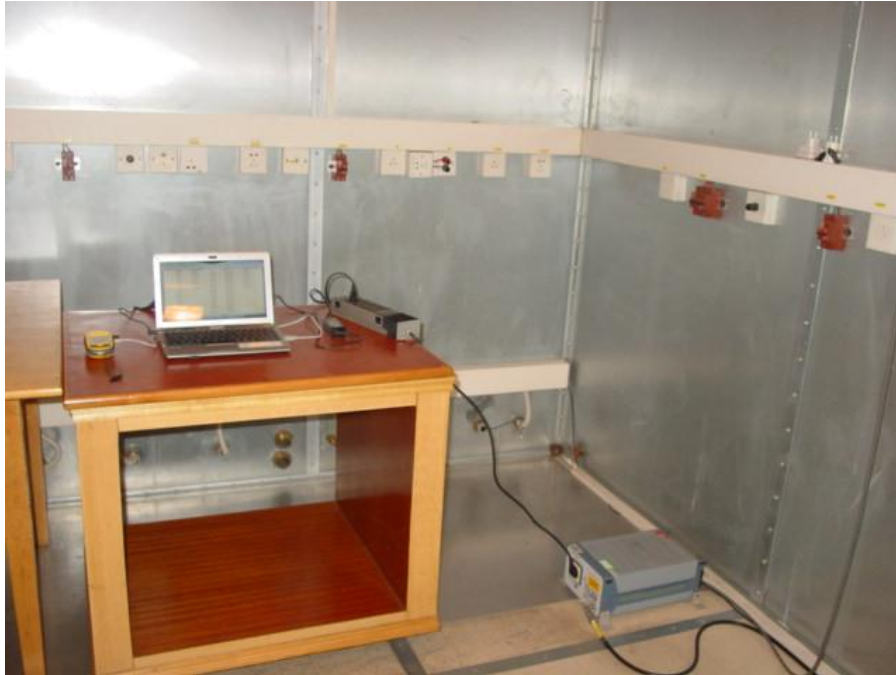
FCC RADIATED EMISSION TEST SETUP-Reading
