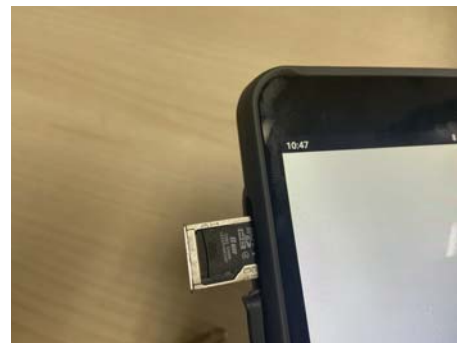
Figure 1-4-8 Installation of Micro SD card
