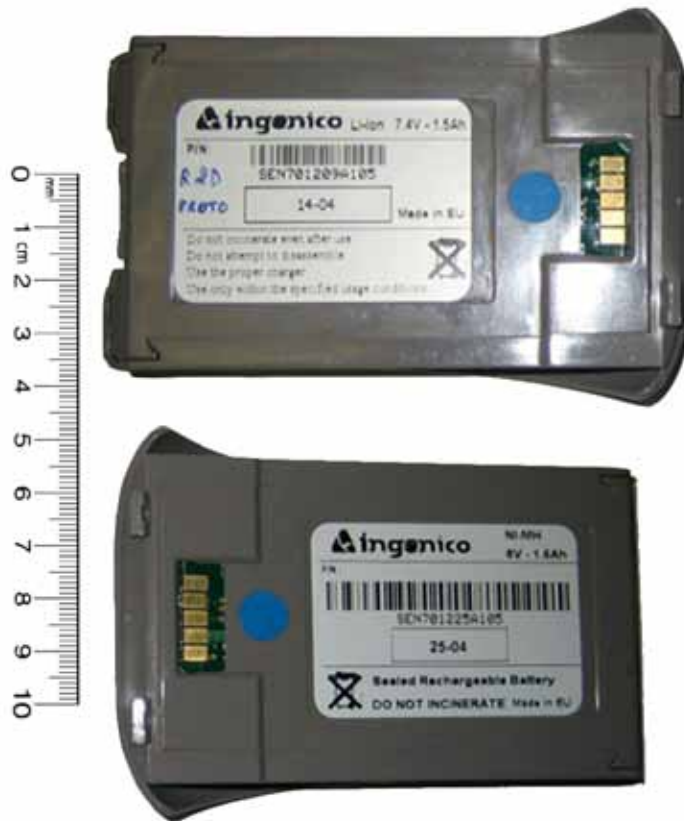
< Rechargeable Li-Ion battery (7.4V 1.5Ah) and Ni-MH Battery (6V 1.5Ah) >
