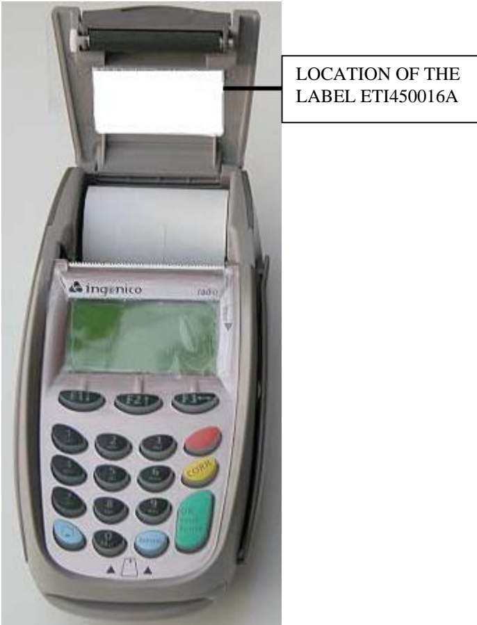
Diagram 2: Position of the product label on i7780 handheld with BTv2.
