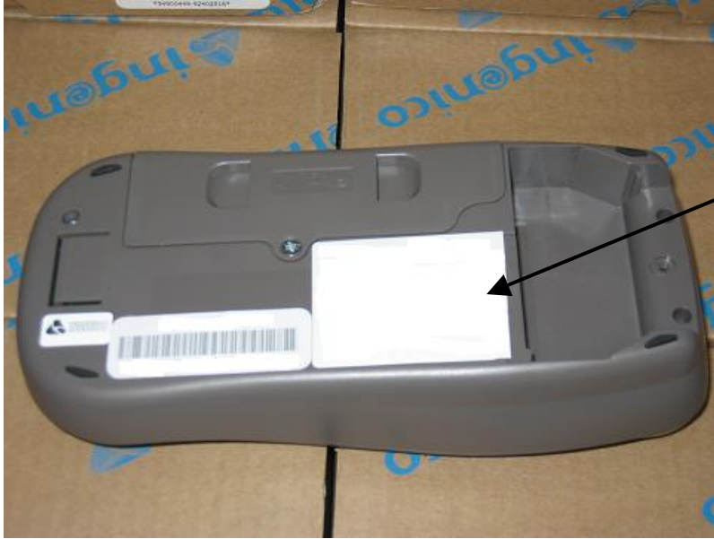
Position of the product label on INGENICO 7780 base
