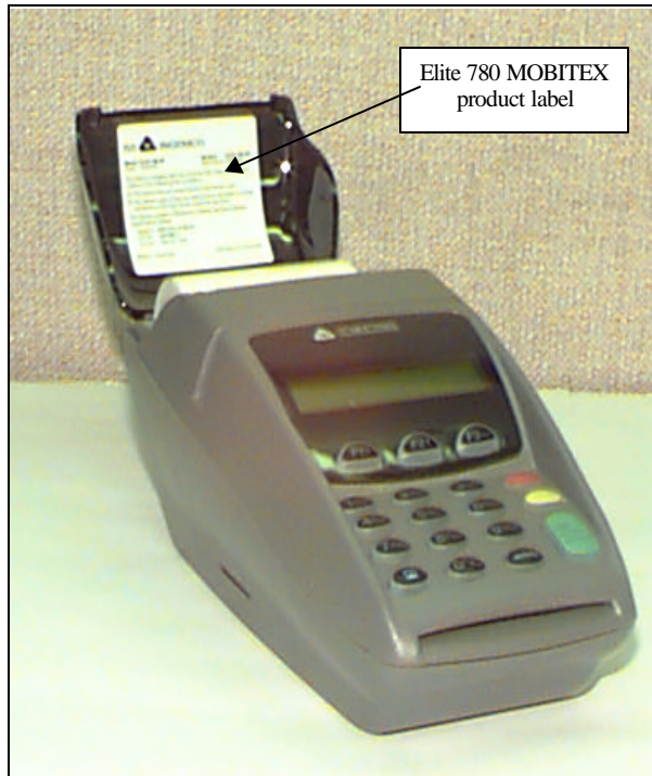
Diagram 2: Position of Product label and Serial number barcoded label on Elite 780 MOBITEK unit.
