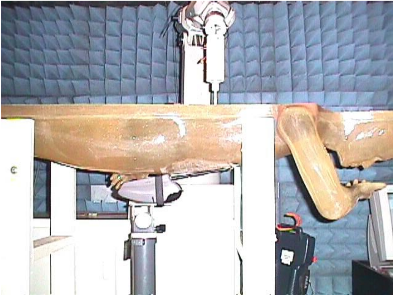
< Overview - Waist with the tip of the antenna in contact with the phantom >
