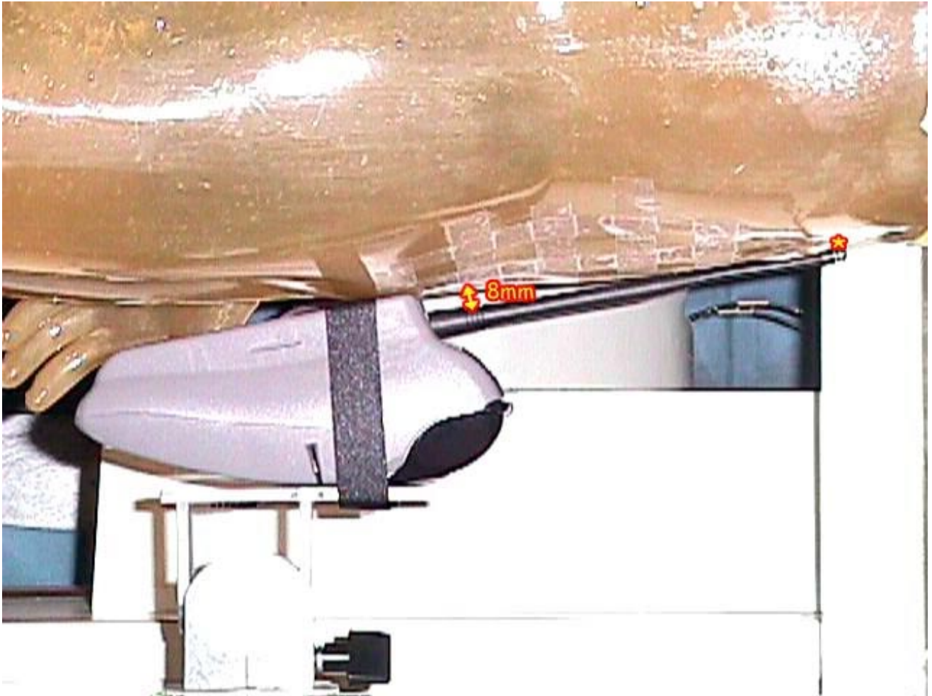
< Close-up view - Waist with the tip of the antenna in contact with the phantom >
