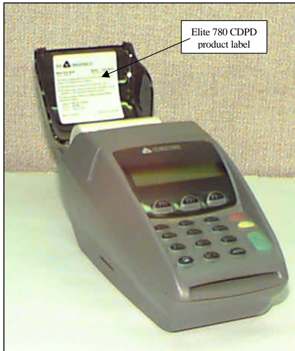
Diagram 2: Position of Product label and Serial number barcoded label on Elite 780 CDPD unit.
