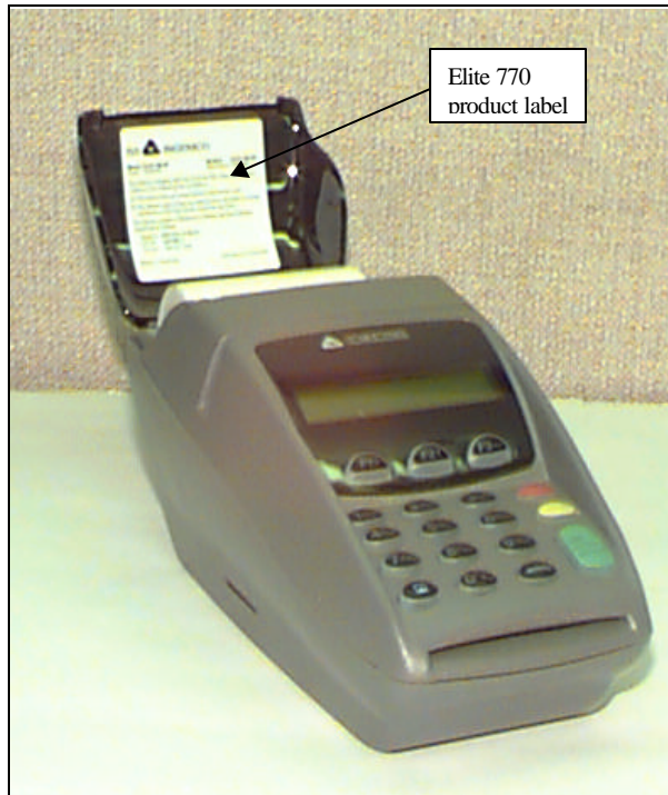
Diagram 2: Position of Product label and Serial number barcoded label on Elite 770 Hand Held unit.
