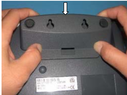
Figure 2: Removing the existing Tyco/Loki Foot
