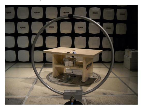
30MHz -1 GHz Measurement setup:
