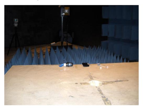
Radiated Band-edge Measurement Setup:
