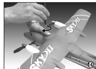
14. Put the main wing on top of the plane and fix it with the \phi 2.0 \times 8 \text{ PB} screws. (Fig.14)
