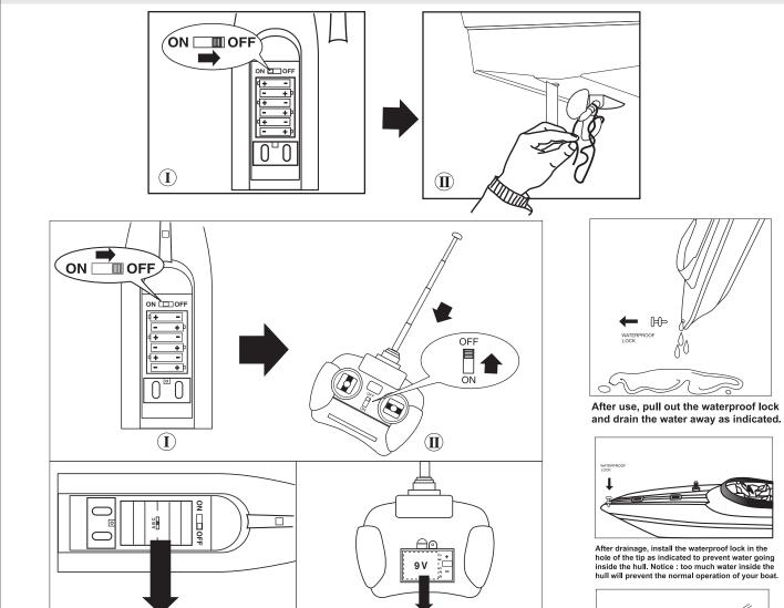
After sailing, switch off the receiver on the boat and
