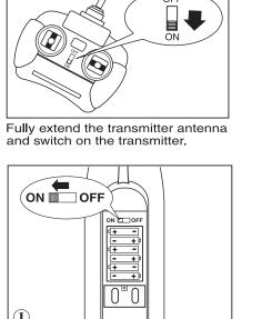
Check whether the propeller and the rudder's turning direction match with the transmitter's input.
