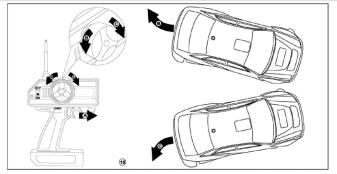
11. when vehicle moves backward,turn the steering wheel counter-clockwise(fig.15), vehicle will turn inward left.
