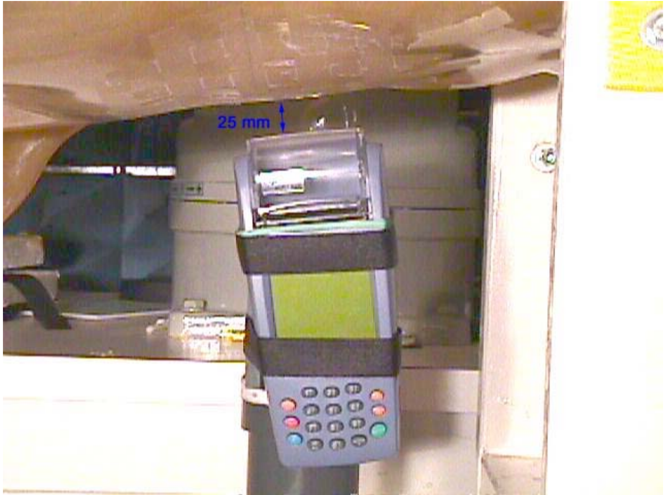
< Top surface of EUT parallel and 25 mm away from the phantom waist – Close-Up View >
