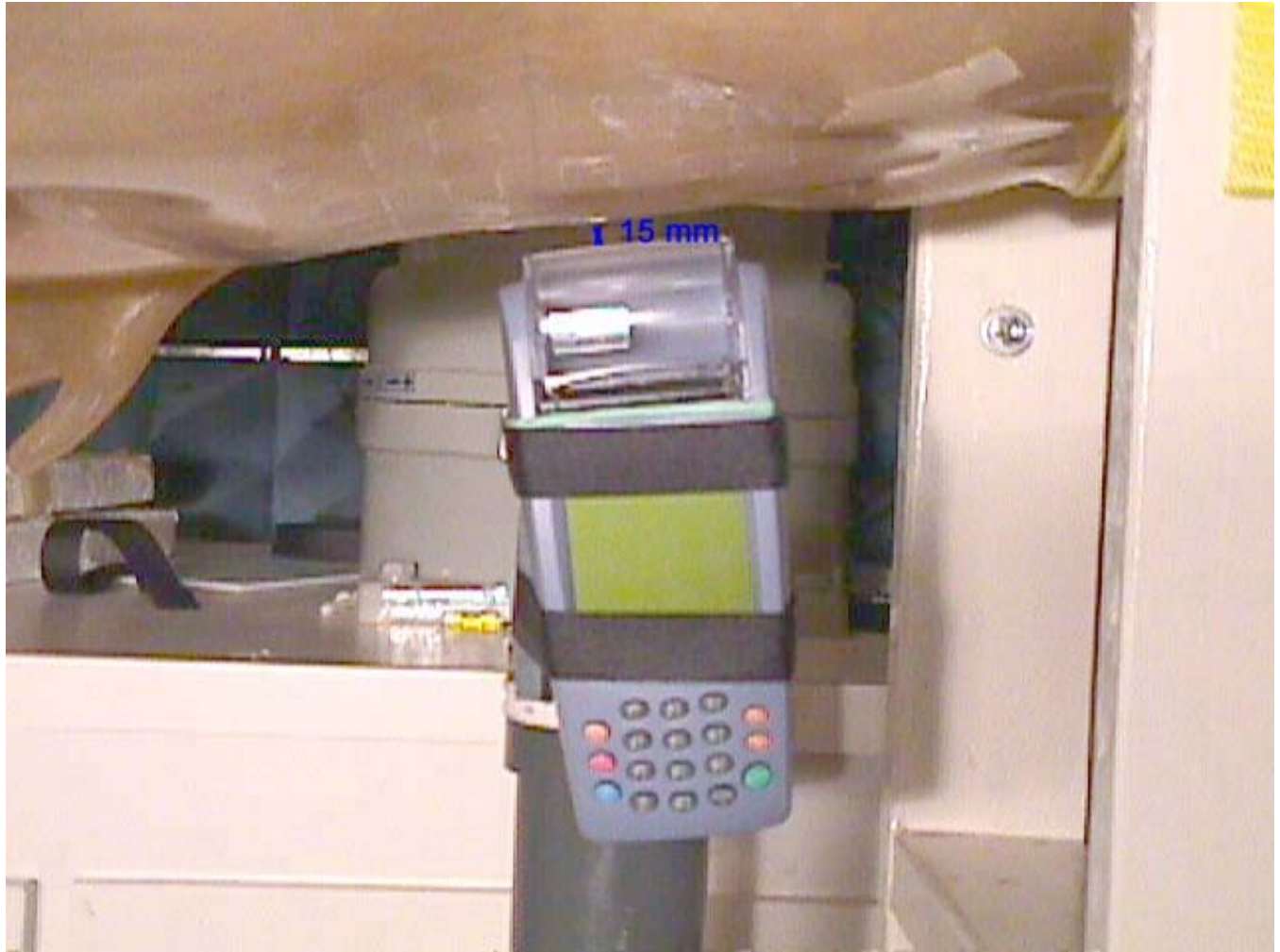
< Top surface of EUT parallel and 15 mm away from the phantom waist – Close-Up View >
