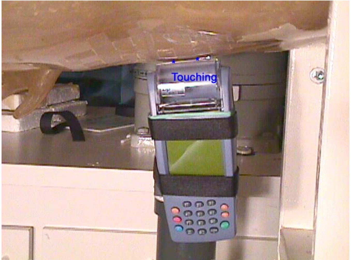
< Top surface of EUT parallel and in contact to the phantom waist – Close-Up View >
