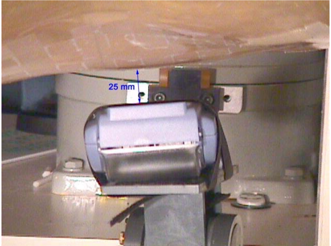
< Back surface of EUT parallel and 25 mm away from the phantom waist – Close-Up View >
