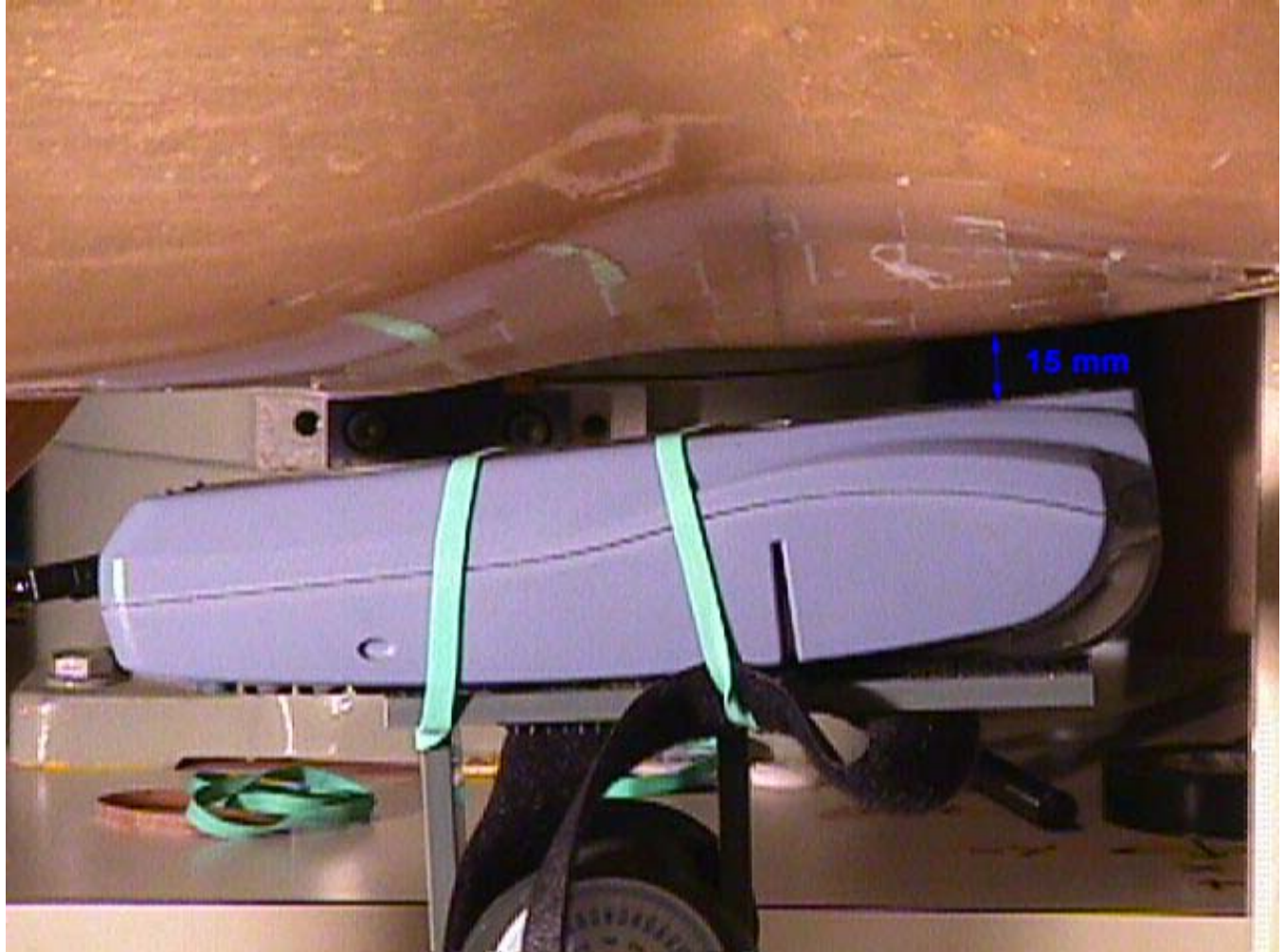
< Back surface of EUT parallel and 15 mm away from the phantom waist – Close-Up View >
