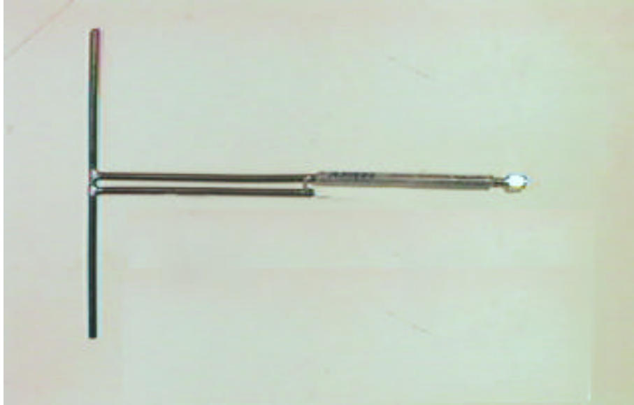
Reference Dipole Antenna Used for ERP Measurement
