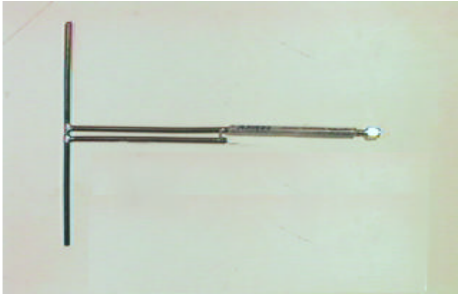
Reference Dipole Antenna Used for ERP Measurement
