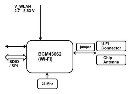
RZ226MS Module mainly consists of Broadcom BCM43362 Wi-Fi device, a 26 MHz crystal, and an on-board chip antenna and a u.FL connector for optional external antenna.
