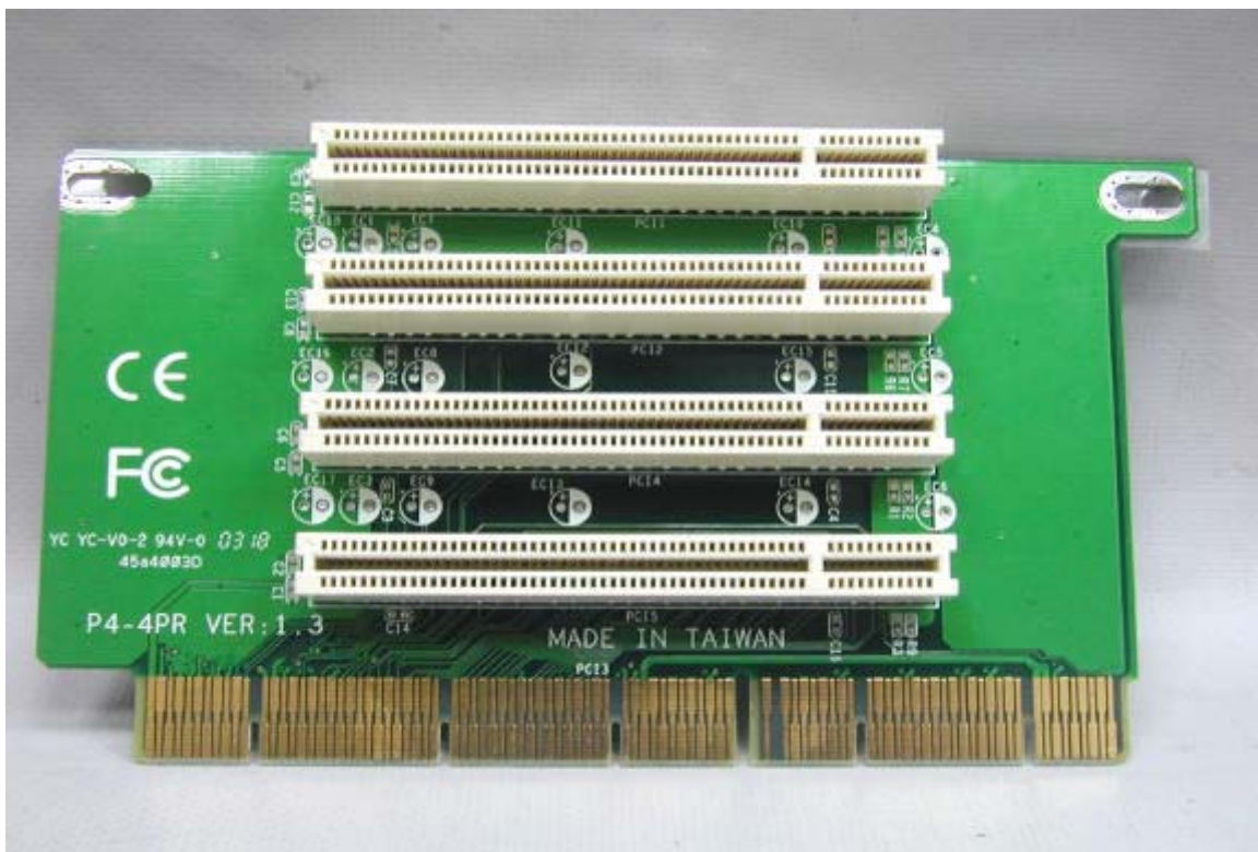
PHOTO. 18. EUT COMPONENT SIDE VIEW (PCI CARD)
