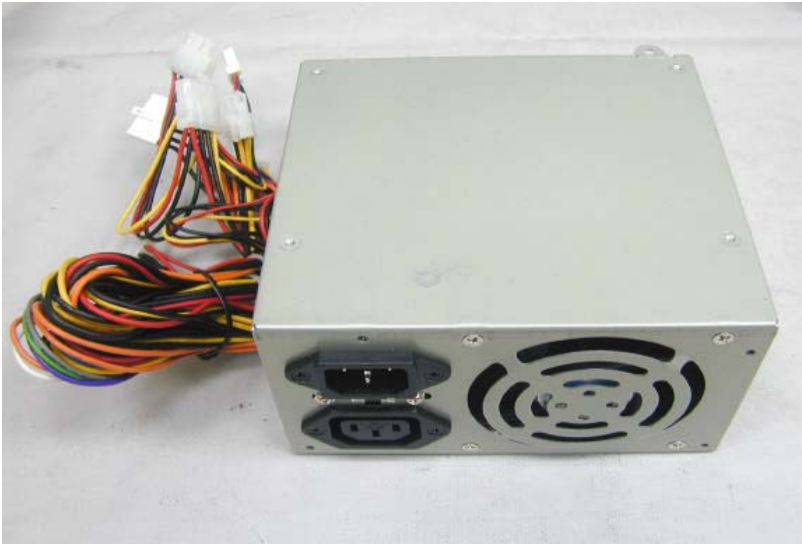
PHOTO. 29. POWER SUPPLY REAR VIEW
