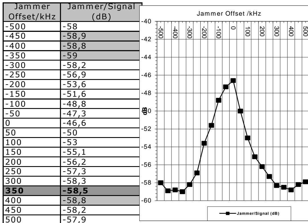
Disregarding the marked data points (-450, -400, -350, 400 kHz) the worst data point is at 350 kHz with a value of -58,5 dB.
