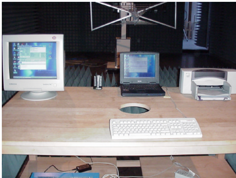
Picture 2 : Test set-up for radiated emissions
