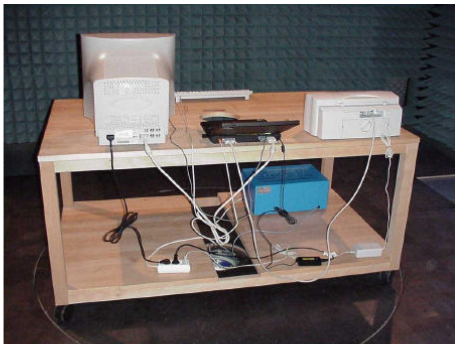
Picture 2 : Setup for radiated measurement, rear view
