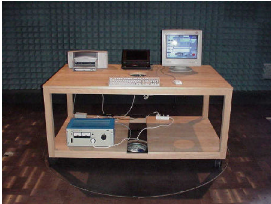
Picture 1 : Setup for radiated measurement, front view
