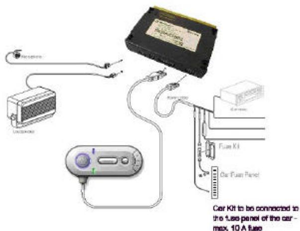
**Figure 1:** Bluetooth Car Kit. The devices not printed in solid black are additional equipment not delivered with the kit.
